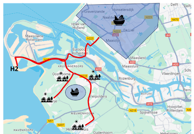
Fig. 7. Schematic of possible district heating near the port of Rotterdam. Fruit icons indicates the greenhouse areas and house icons indicate house areas. The red lines indicate the tracés for transport lines.
