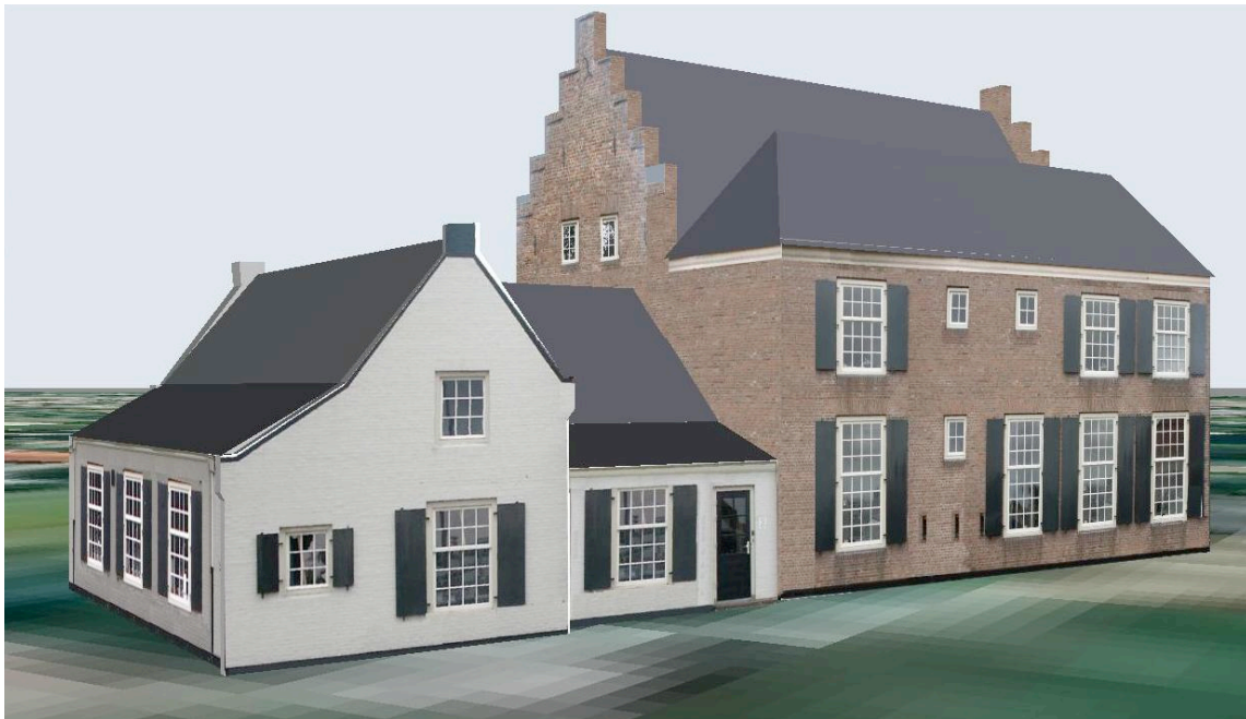
Figure 4: Parametric models and horizontal extrusions combined
