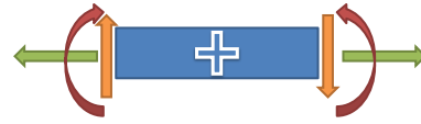
Figure 8.2: Positive direction of normal (green) and shear forces (orange) and moments (red).
