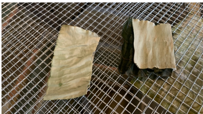
Glued sheet structure (left), Corrugated fiberboard sample (right)
