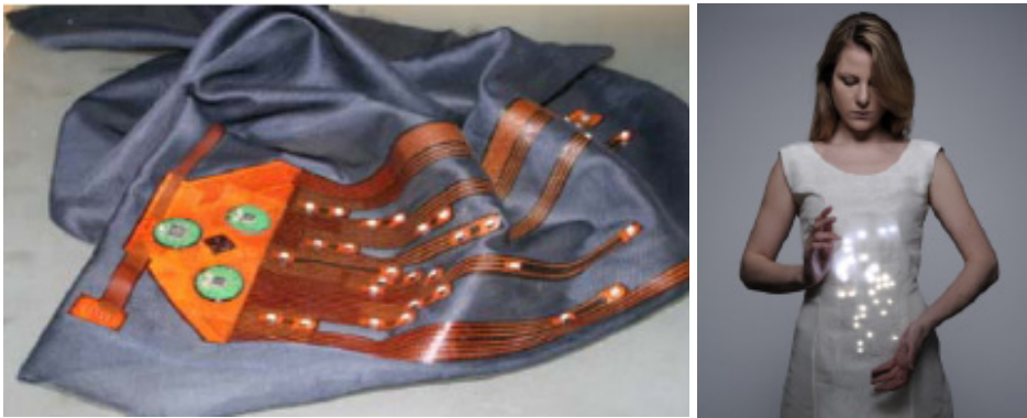
Figure 2-20. Stretchable electronic system laminated to fabrics [2.12]
