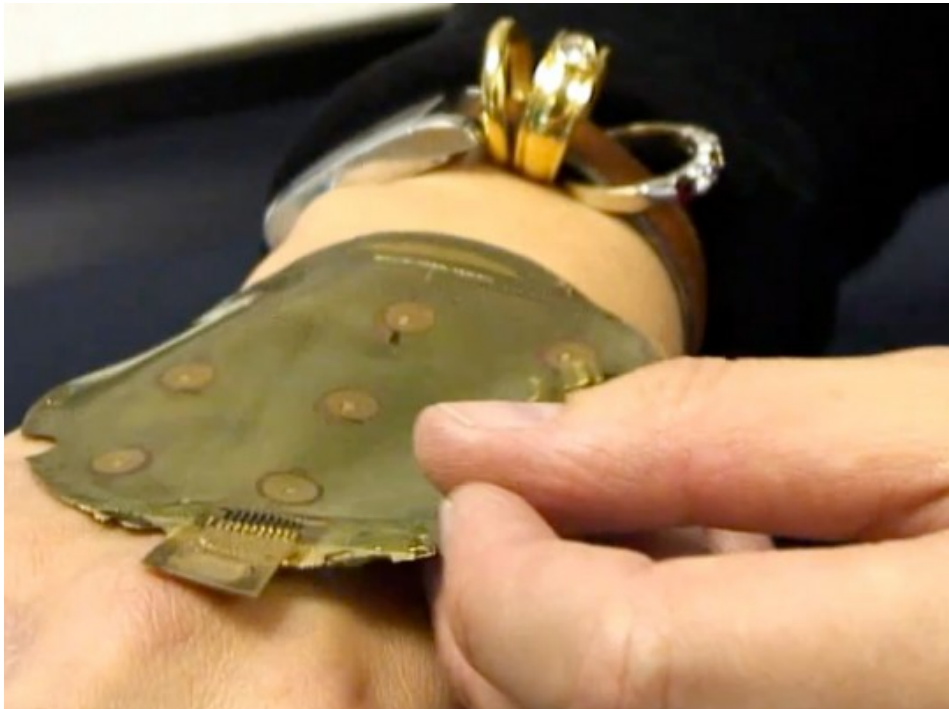
Figure 1-2. Artificial electronic skin being developed by Nokia and Cambridge University [1.2].
