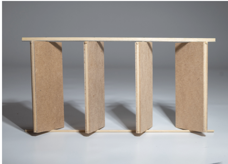
Pivoting walls that open and close depending on the need; when closed - fully sealed
