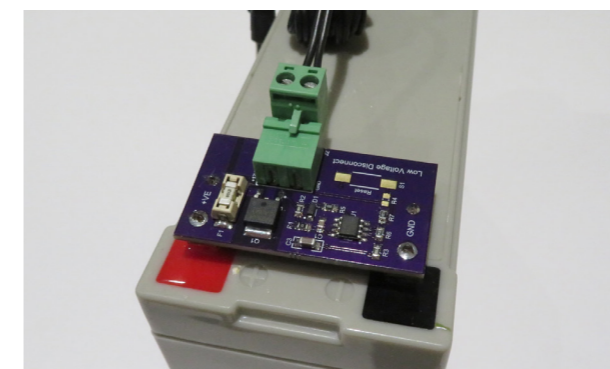
Figure 37: PCB with safety circuit, designed by C. Peacock [96]
