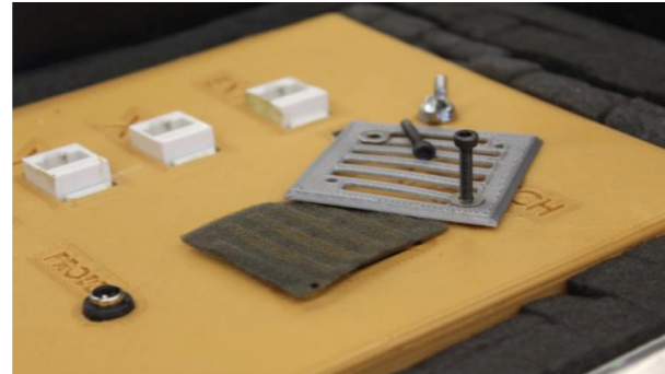
Figure 22: Kijenzi's method for stopping dust included a simple dust filter [10]
