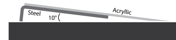
Figure 64: Final attempt uses an acrylic-steel wedge under a 10 degree angle
