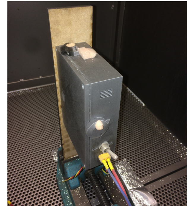
Figure 53: Final dust test setup of the enclosure in a sandblasting chamber
