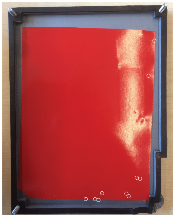
Figure 55: Results from the dust test. White circles indicate penetrated particles
