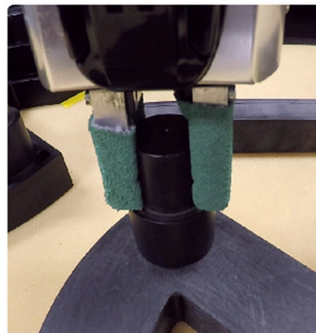
Figure 18. An example of using DMPs in assembly tasks (e.g., peg-in-the-hole) (Kramberger et al., 2016b).
