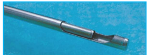
Figure 5: The tip of the hysteroscopic tissue removal device, showing an outer tube with a side-facing cutting window and a tubular cutting blade that can rotate and reciprocate inside the outer tube [39].
