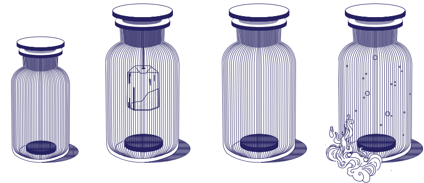
Step 1. Inherent smell Step 2. Absorption Step 3. Diffusion Step 4. Heat and humidity /Jar and material sample/ /Jar, rosebuds in a tea bag and material sample/ /Jar and material sample/ /Jar, water drops, warm water, and material sample/
