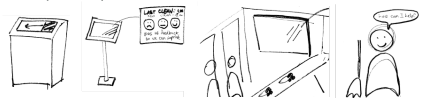
Figure 14: Most promising ideas. From left to right: automatic sliding hygienic lid for bins, tablet to give and receive feedback on the toilets, feedback screens with entertaining informative waiting videos and the cleaner as host.
