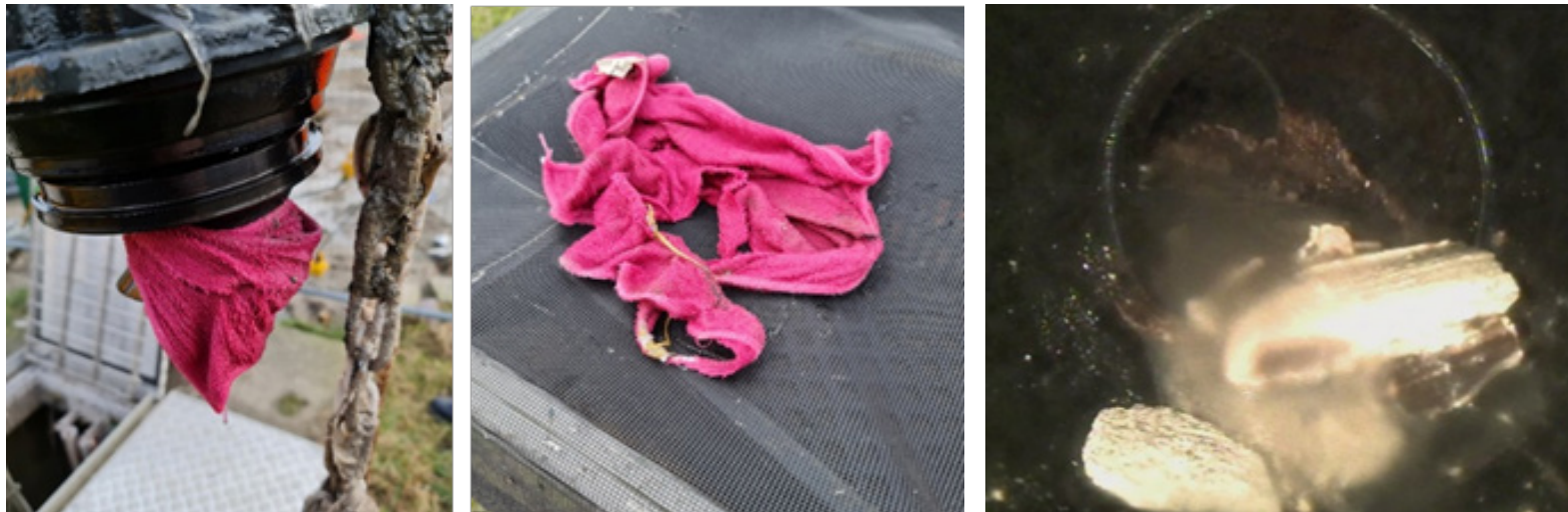
Figure 3: Obstructions in wastewater pumps. Above obstructions by paper, below obstruction by towels and struvite scale
