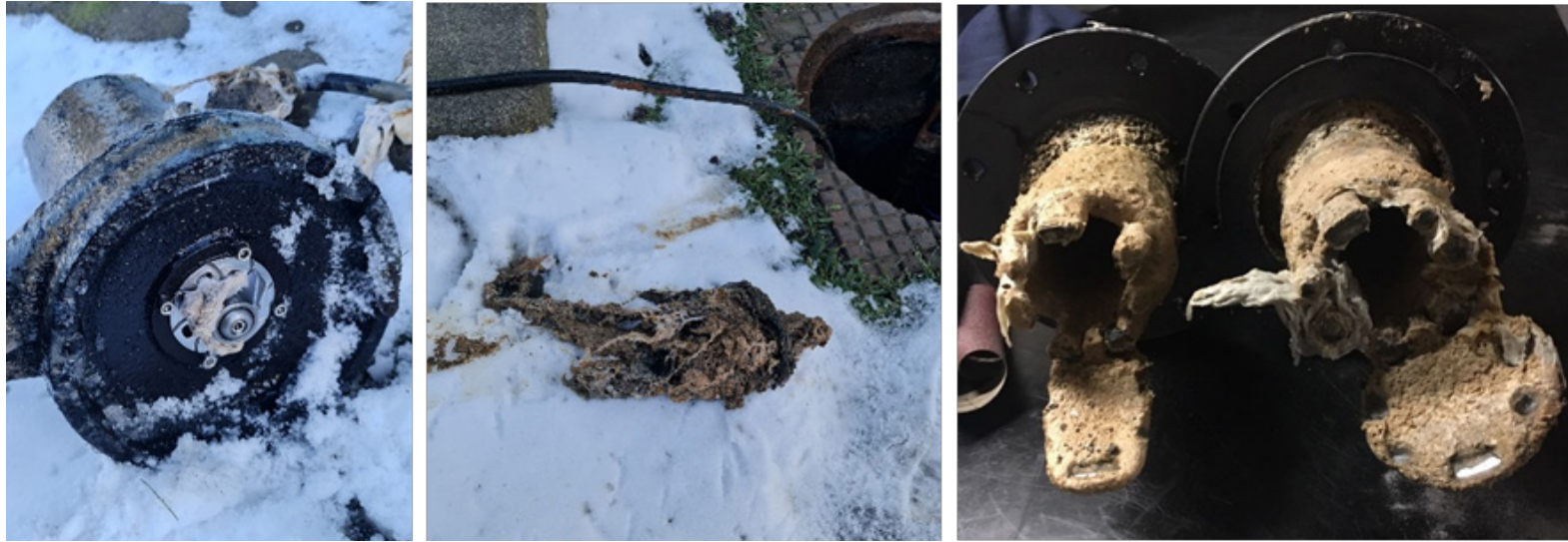
Figure 3: Obstructions in wastewater pumps. Above obstructions by paper, below obstruction by towels and struvite scale
