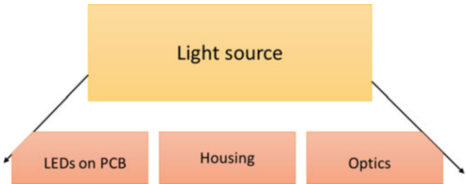
Fig. 13.15 Sub-systems in the light source function
