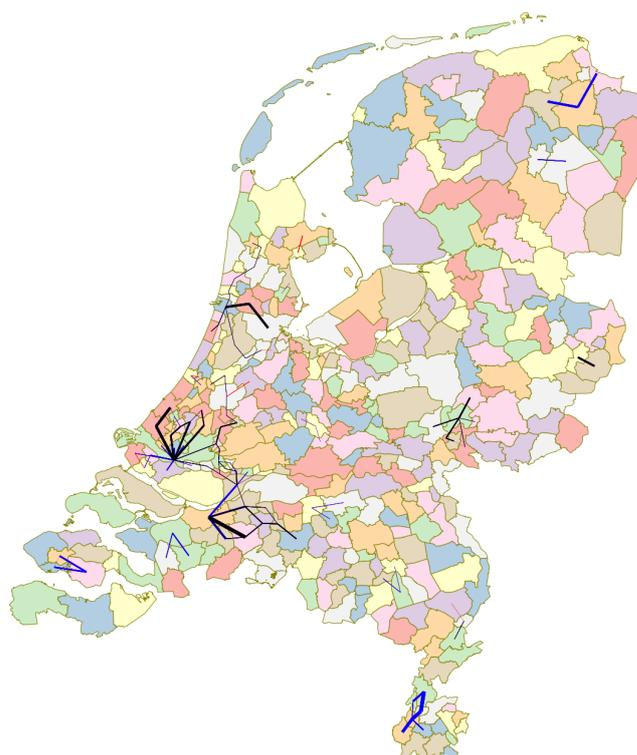
Figure 5.2: Scenario40% - Expansion of pipeline networks over the years (black, 2020; blue, 2030; red, 2040)
