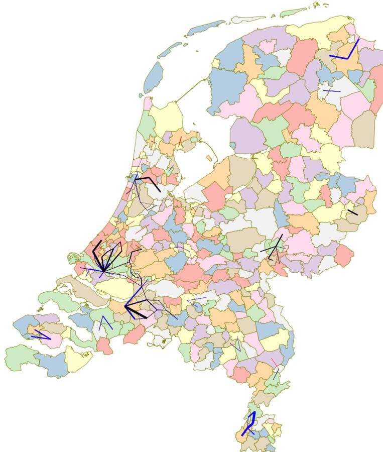
Figure 4.16: Expansion of pipeline networks over the years (black, 2020; blue, 2030; red, 2040)
