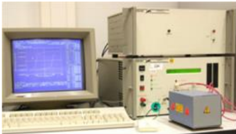
Fig. 2.9: Piezoelectric hysteresis and polarization fatigue measurement set-up
