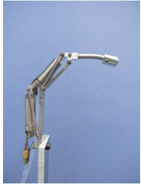
Figure 4.4 Two fingers with identical parameters were made: the pulley finger (left) and the cylinder finger (right). The only parameter that differed was the transmission principle. The same springs were used in an identical configuration in each finger, to extend the finger.
