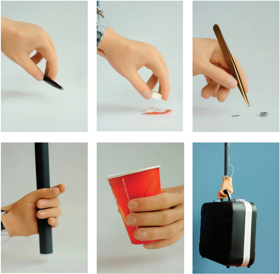
Figure 7.4 The underactuated hand adapts to the shape of the grasped object, without using any sensor and by using only one control signal. The hand can perform the two basic grasp patterns: precision grip and power grip. The hand can pick up small objects with the precision grip (top left and middle). The feedback allows precision tasks, like handling a pair of tweezers (top right). The hand can hold cylindrical objects with the power grip (below left). The little finger can be used to support the object, e.g. a cup (below middle). The power grip can also be used to carry a load in a horizontal position, e.g. the handlebar of a suitcase (below right).
