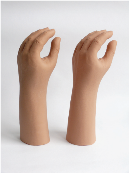
Figure 5.1 Two of tested cosmetic gloves: The PVC glove (left) and the silicone glove (right). The gloves were identical of size, shape and texture. Only the material differed. The fingers are slightly flexed in their neutral position.
