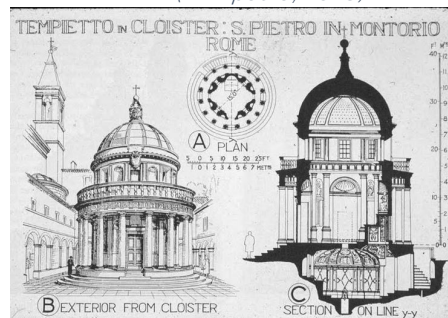
Figure 14 Perspective, floorplan and section of the Tempietto. (Whoop, 2011)
