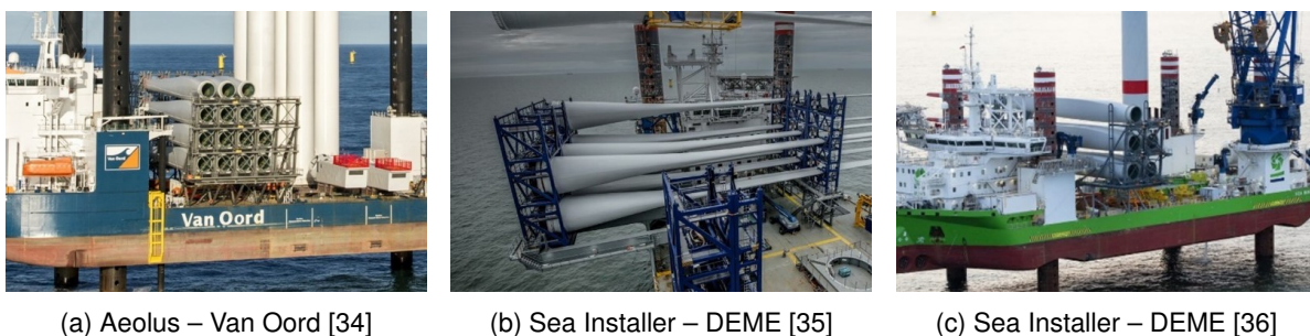
Figure 3.5: Current methods of storing wind turbine blades on deck of a jack-up vessel
