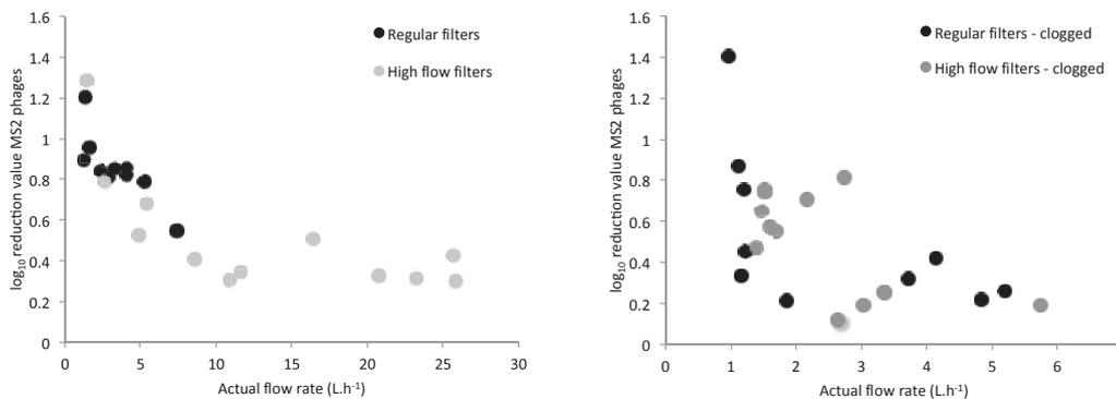
Fig. 7. MS2 bacteriophages removal immediately after scrubbing of clogged filters (left) and again clogged filter (right) related to actual flow rate.
