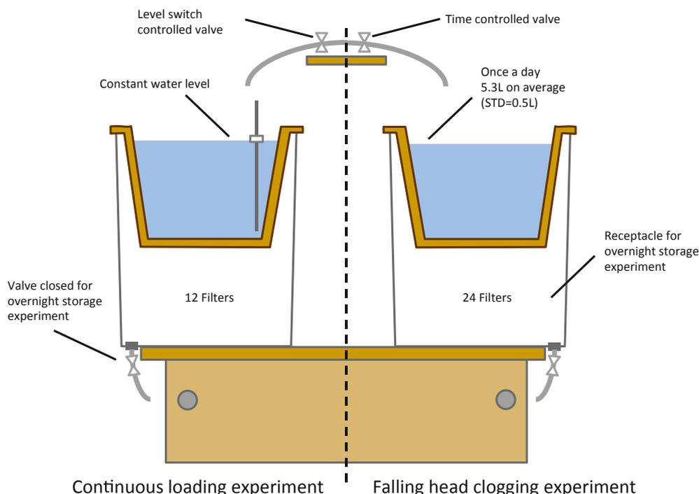
**Fig. 2.** Experimental set-up for (right) falling head clogging experiment and (left) continuous loading experiment. Receptacle and valve for overnight storage experiment are also indicated in the figure.
