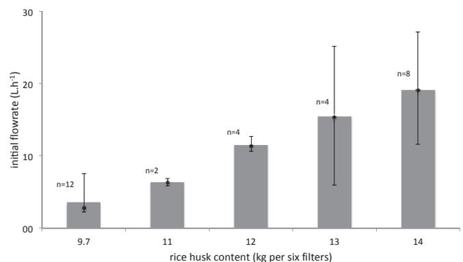
Fig. 3. Relationship between initial, clean filter flow rate and rice husk content of 9.7 (regular), 11, 12, 13, and 14 kg.
