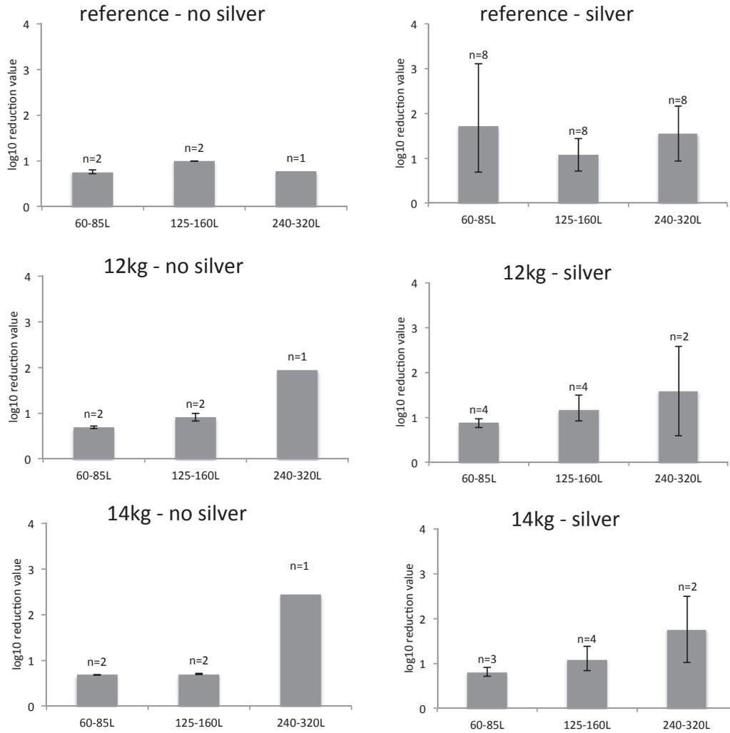
Fig. 6. LRV in relation to the throughput of water during the long-term falling head experiment without (left row) and with (right row) Ag application for the reference filters and high flow filters with either 12 or 14 kg rice husk.
