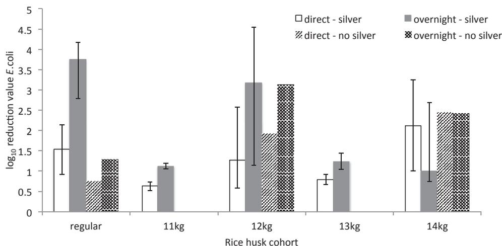
Fig. 10. *E. coli* LRV after overnight storage, throughput <300 L, black circles indicate result of sample taken from filter without Ag application.
