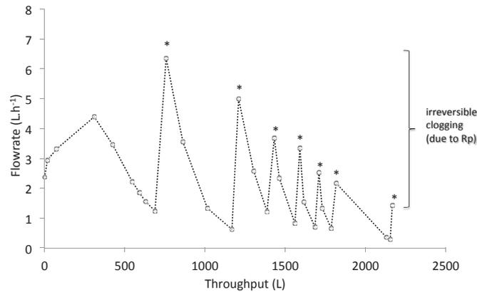
Fig. 8. Flowrate development caused by resistance build-up for a 12 kg pot filter (\* indicates a scrubbing event).
