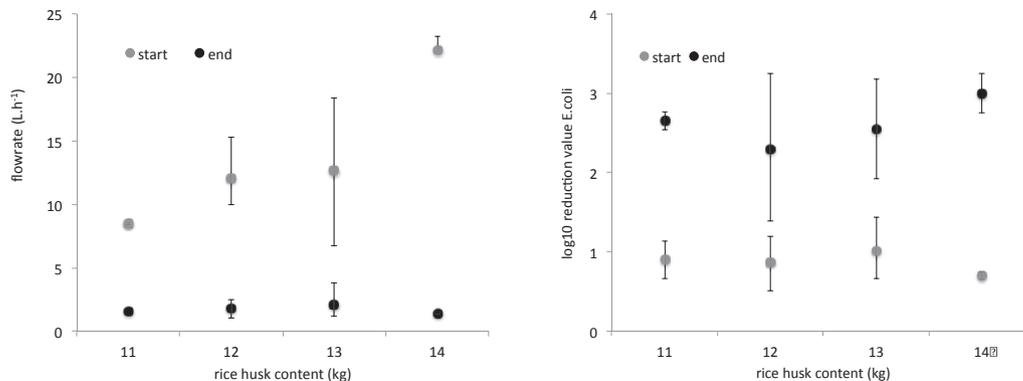
Fig. 9. Flow rate (left) and log<sub>10</sub> reduction value (right) per rice husk content cohort (11, 12, 13 and 14 kg) at start and at end (400 h, >1700 L) of the continuous loading experiment. Flow rates were determined at the moment of the *E. coli* spike, which was before a scrubbing event, i.e. flow rates are lower than after scrubbing.
