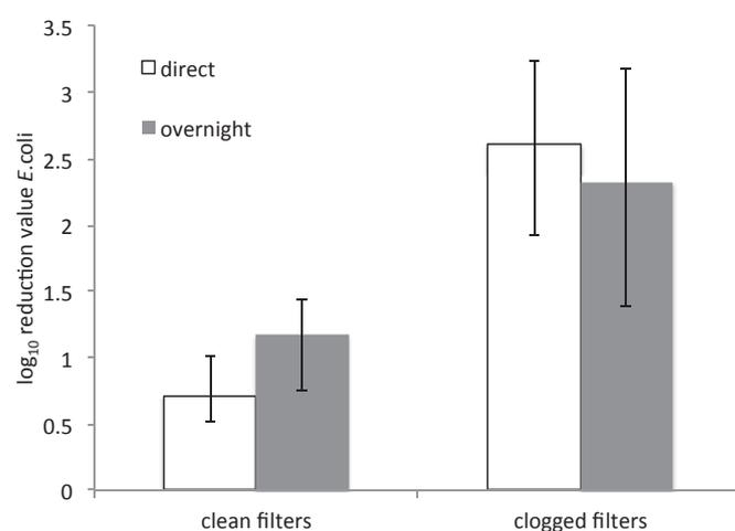
Fig. 11. *E. coli* LRV after overnight storage, in clean and clogged filters in the continuous loading high flow filters.
