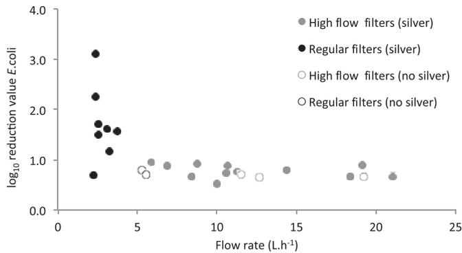
Fig. 4. Clean filter  $\log_{10}$  reduction values for *E. coli* per initial flow rate.
