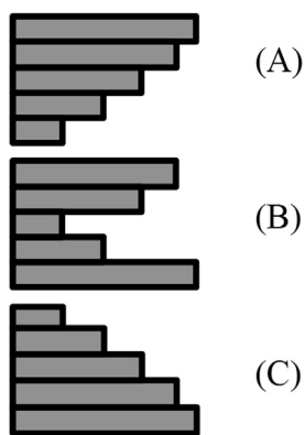
Fig. 3. Schematic of spatial ordering of layer permeabilities.
