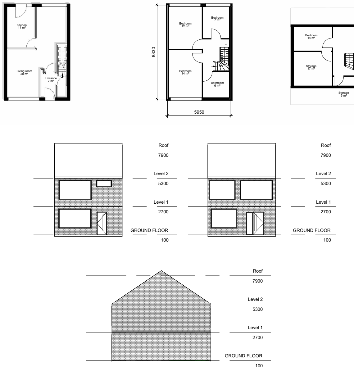
Figure 18. Floor plans and elevations of a typical 60s terraced house in the Netherlands (created by author).
