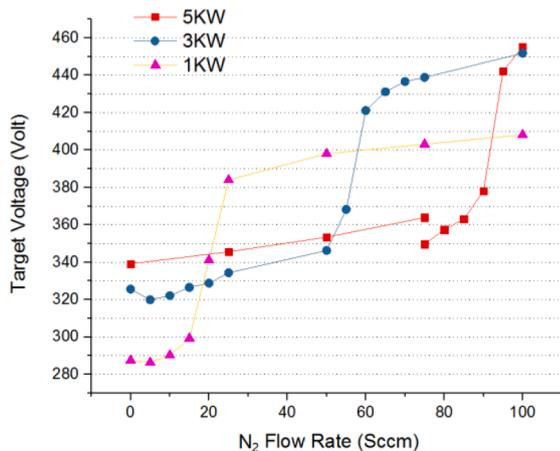
Fig. 8. Discharge voltage as a function of  $N_2$  flow rate at target powers of 1 kW, 3 kW and 5 kW. The platen temperature is 350 °C and the Ar flow rate is 100 sccm.
