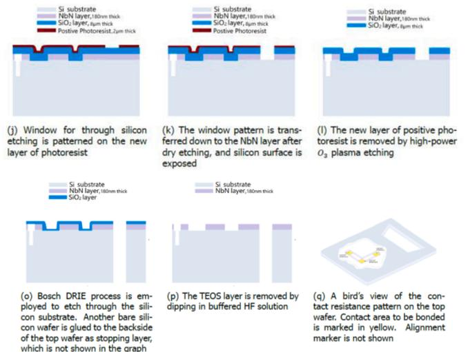
Fig. 6. Fabrication of contact resistance pattern on the top wafer.
