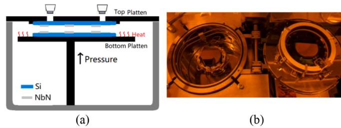
Fig. 4. (a). Illustration of the wafer bonder (b) Top and bottom wafers loaded on the platens.
