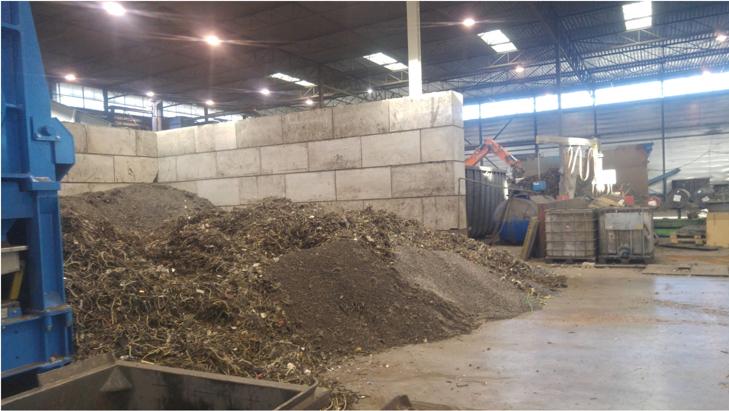
Figure 25: Shredded power cable at a cable recycling facility
