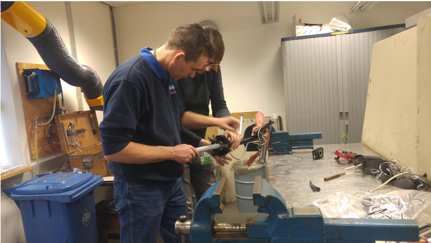
Figure 26: Inspection and dismantling of a damaged medium voltage power cable at Alliander
