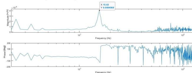
(b) Frequency response of N2 with silicone coating in air
