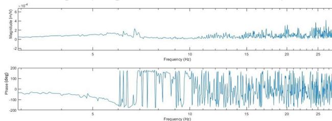
(c) Frequency response of N2 with silicone coating in water
