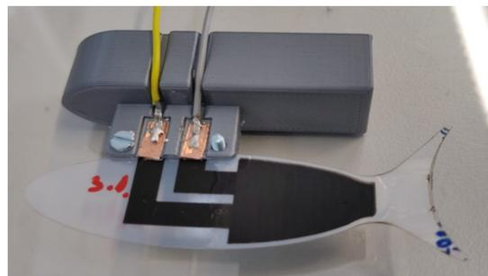
Fig. 1: PVDF-based inkjet printed robotic fish
