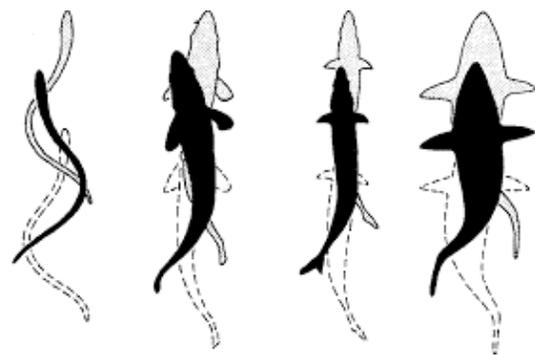
Fig. 5: Variations from undulatory to oscillatory motion in BCF swimming form. Left to right: Anguilliform, Subcarangiform, Carangiform, Thunniform [12]
