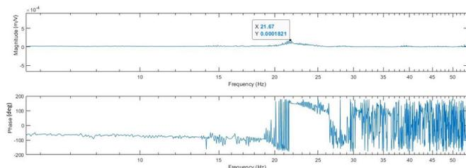
(b) Frequency response of N5 with silicone coating in air
