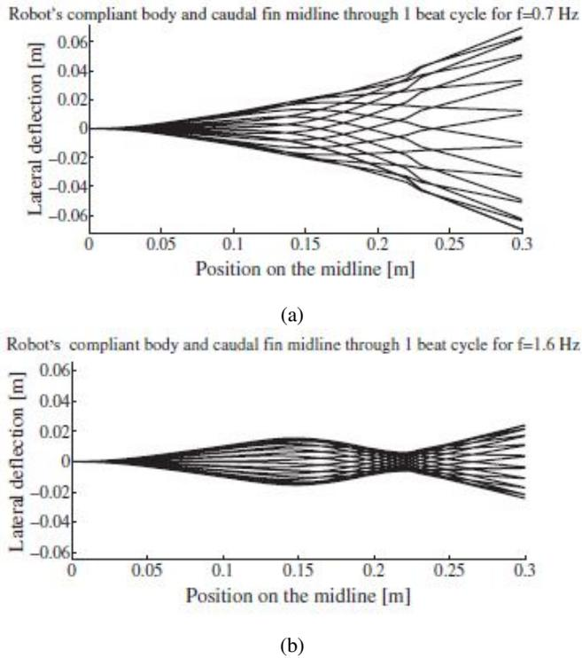
Fig. 12: Robot's compliant body and caudal fin midline for different frequencies [41]
