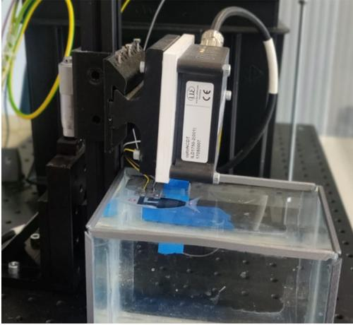
Fig. 12: Experiment set-up to evaluate the operating frequency in water
