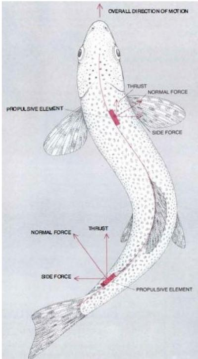
Fig. 6: With the propulsive wave passing down the body, forces act on segments by moving each element laterally and accelerating the water nearby. The normal force exerted on the water has two components: side force and thrust in the direction of overall motion. The magnitude of thrust contributed by each body element increases towards the tail. [23]
