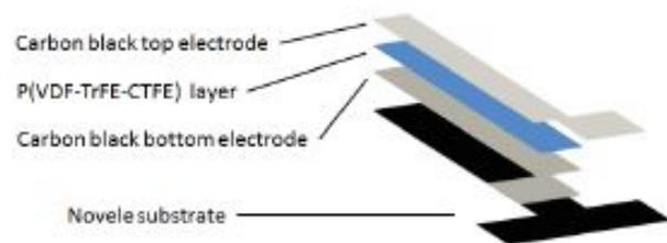
Fig. 9: PVDF actuator in layered structure [34]
