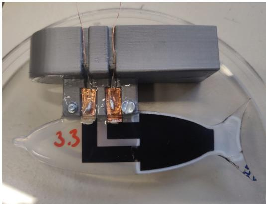
Fig. 24: Altered copper wiring routed onto the float
