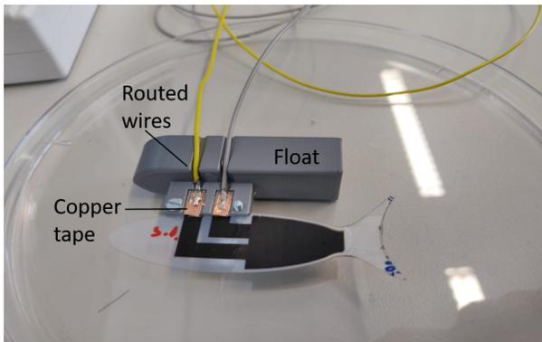
Fig. 8: Actuator attached to the float with established electrical connections
