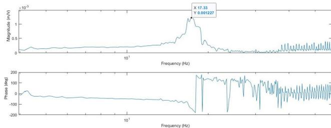
(a) Frequency response of P2 without coating in air
