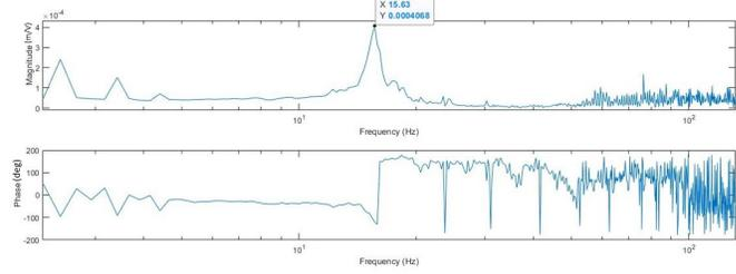
(b) Frequency response of N2 with silicone coating in air
