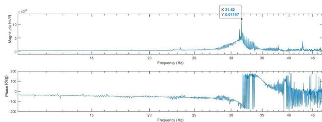
(a) Frequency response of N5 without coating in air
