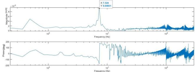
(b) Frequency response of P2 with silicone coating in air
