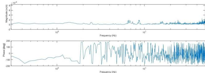
(c) Frequency response of P2 with silicone coating in water
