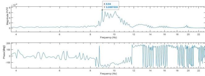
(a) Frequency response of K4 with silicone coating in air
