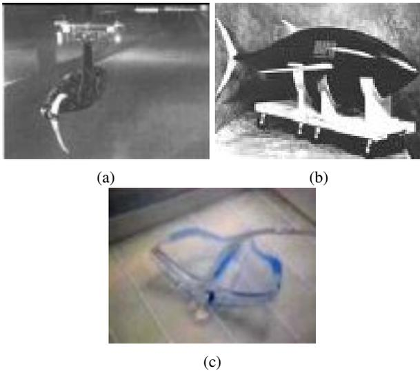
Fig. 2: Underwater robots using different actuators (a) DC servo motor actuated Robotuna (b) hydraulic cylinder actuated VCUUV (c) pneumatic actuated Manta Robot [12]
