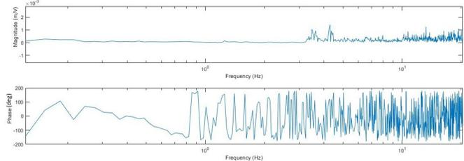
(b) Frequency response of K4 with silicone coating in water
