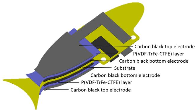
Fig. 4: Schematic representation of a bi-morph actuated robotic fish
