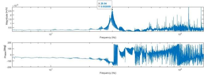
(b) Frequency response of N4 with silicone coating in air
