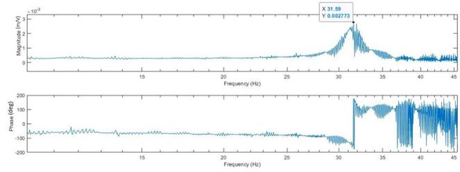
(a) Frequency response of N4 without coating in air
