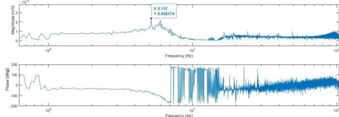
(c) Frequency response of N3 with silicone coating in water
