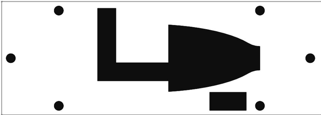
Figure C.3: Left side top electrode pattern
