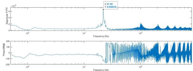
(b) Frequency response of N3 with silicone coating in air
