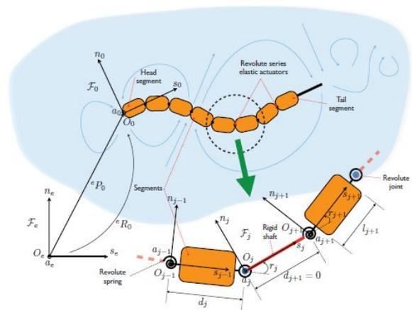
Fig. 11: Schematic representation of internal kinematics of fish-like swimming [43]
