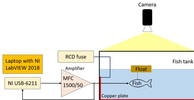
Fig. 13: Experiment set-up to evaluate the performance of the robotic fish
