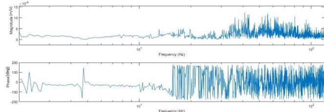
(c) Frequency response of N4 with silicone coating in water
