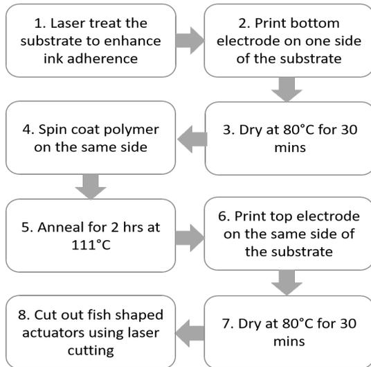
Fig. 7: Manufacturing steps for producing inkjet printed unimorph actuators
