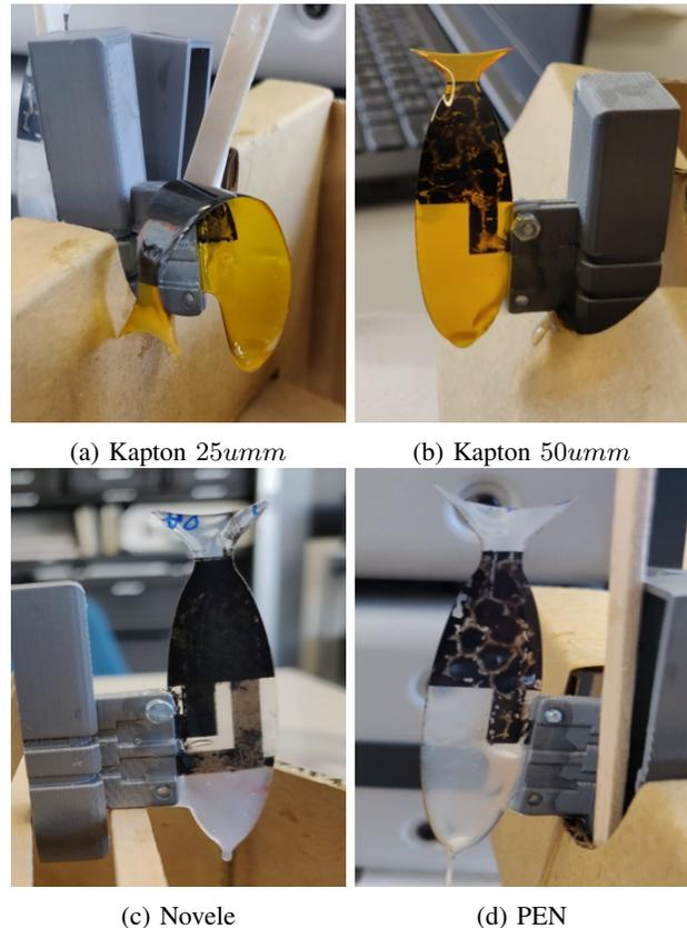
Fig. 9: Substrate samples tested by dipping them in silicone
