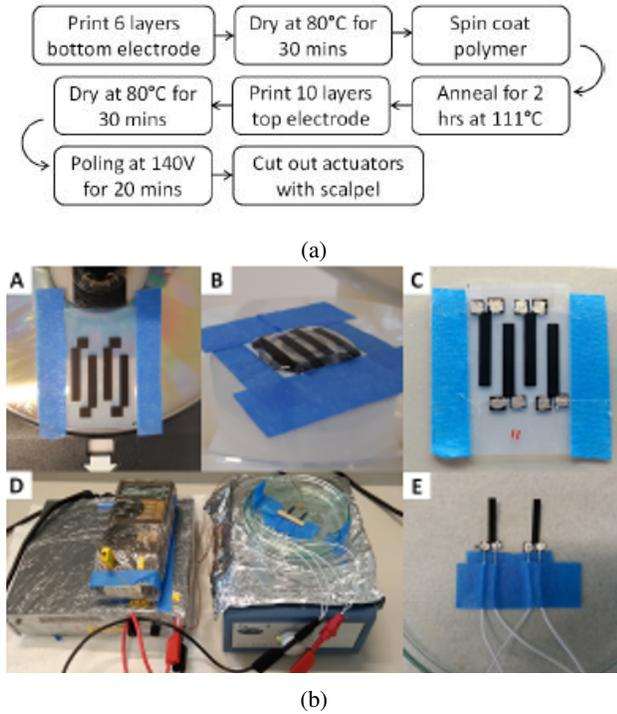
Fig. 10: (a) Steps involved in manufacturing PVDF actuator (b) Making of P(VDF-TrFe-CTFE) actuator [34]
