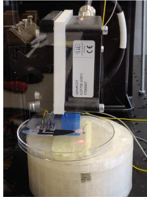
Fig. 11: Actuator being tested in air to evaluate operating frequency
