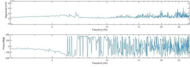
(c) Frequency response of N2 with silicone coating in water
