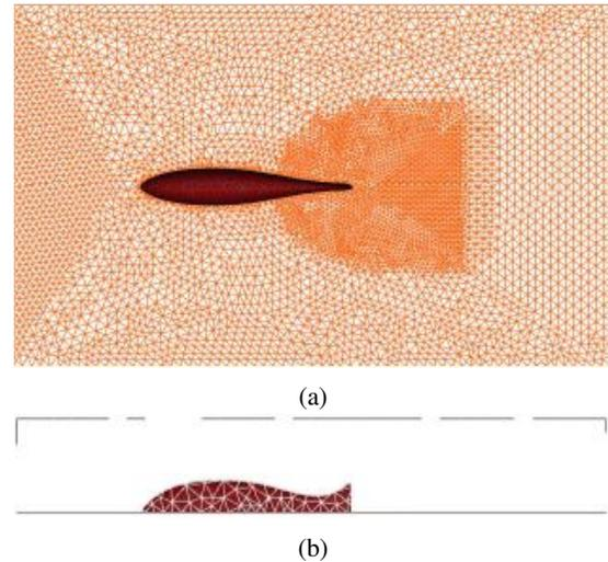
Fig. 13: (a) Top view of fluid domain (b) Side view of fluid domain with flow from left to right, robot has a wall boundary while others are slip boundaries [42]
