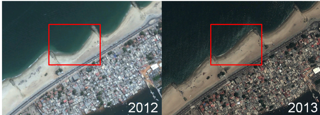
Figure 4.4: The coastline change of the area between the groynes in the red box gives an indication of the minimal required LST in this area.
