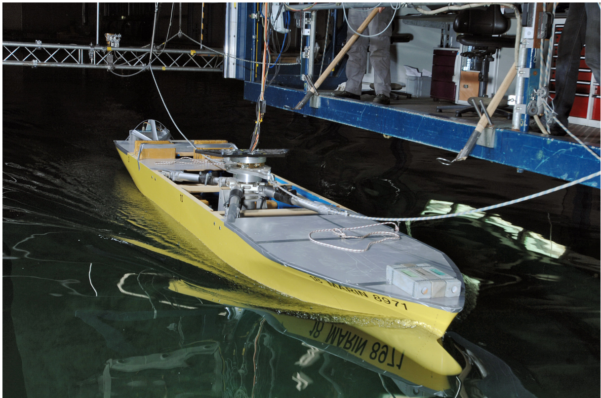
Figure 6.3: HTC ship model during free sailing manoeuvring test
