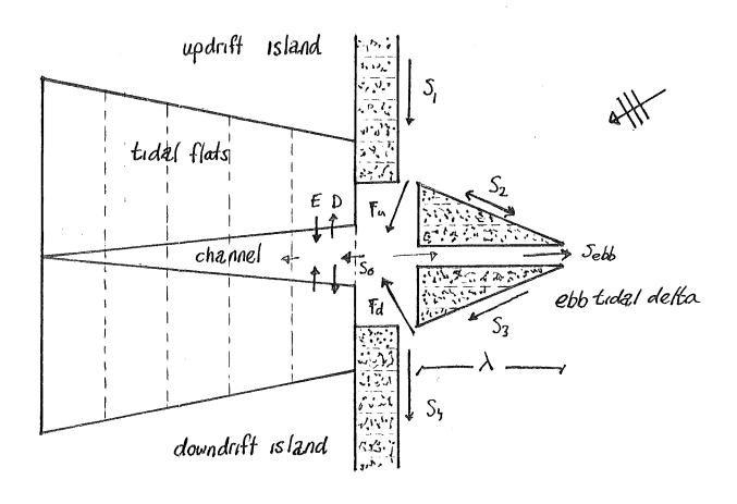
Figure 2: Schematized planform
