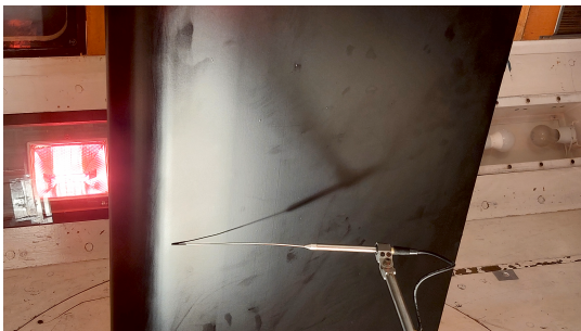
Figure 5.2: Model with microphone along the suction side (left) and the infrared image with the microphone (right)
