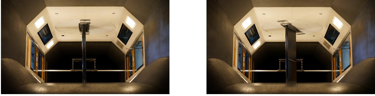
Figure 3.8: Difference in exposed surface area of the V3 model in the LTT at \alpha = 0^\circ (left) and \alpha = 25^\circ (right)
