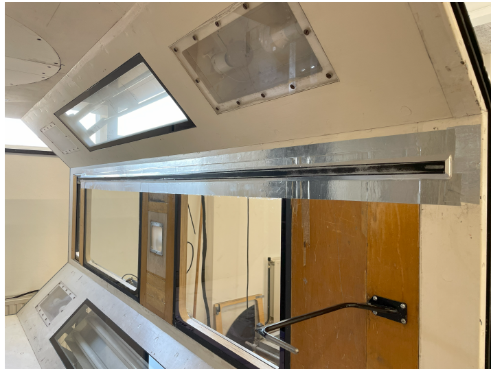
Figure 4.1: Pressure strip mounted on the side of the wind tunnel
