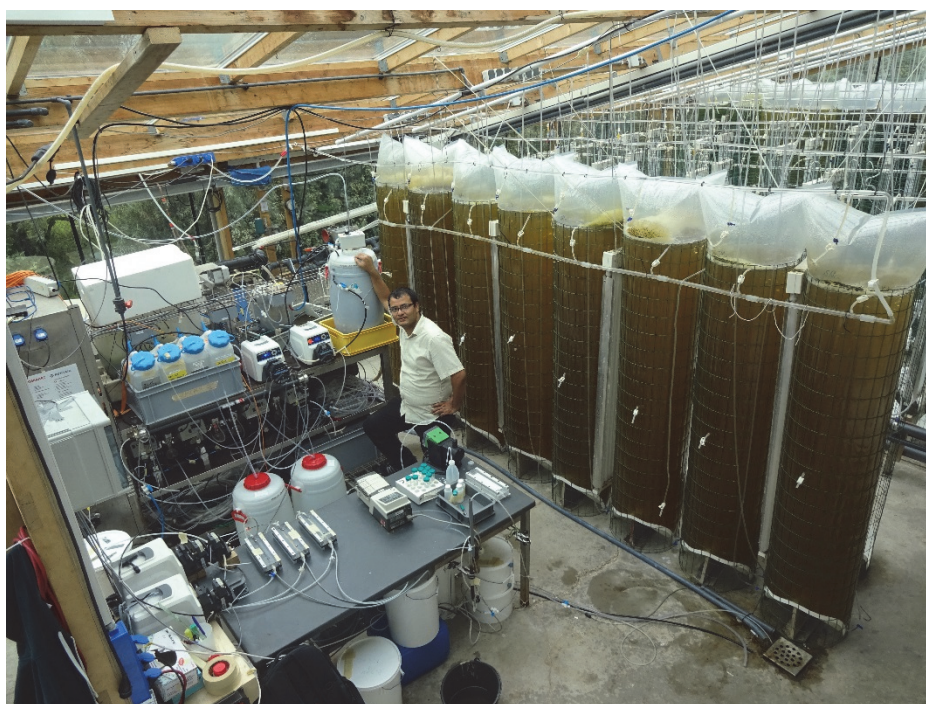
Supplementary Figure S.5.3: General overview of a pilot plant in Zeeland, Jacobahaven, the Netherlands. The large plastic bags are the algal culture of marine diatom Chaetoceros affinis
