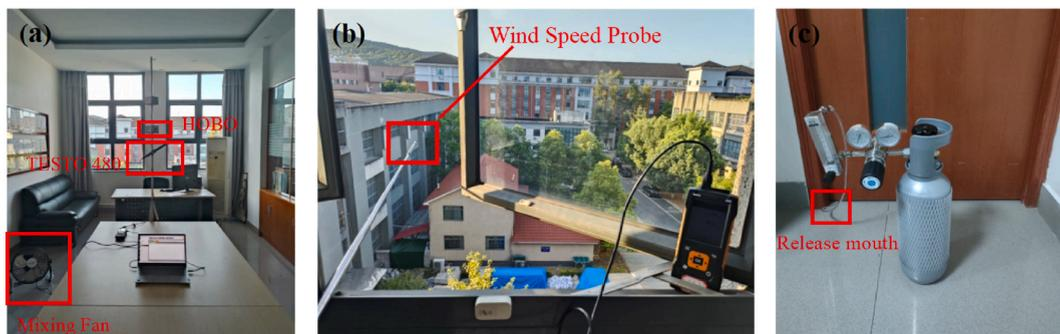
Fig. 3. Layout of the tested spaces: (a) Global view, (b) Outdoor wind speed measurement location, and (c) CO<sub>2</sub> release location.
