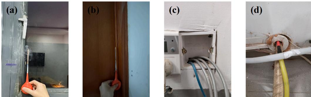
Fig. 5. Approximate detection of air leakage paths: Smoke pen test: (a) Exterior window and (b) Interior door; Direct observation: (c) Socket base and (d) Through-wall pipeline.
