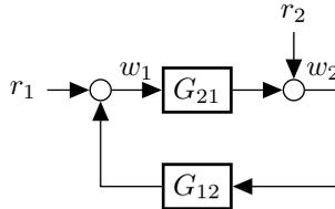
Figure 2.7: Closed-loop system considered by Willems (1971) when discussing well-posedness.
