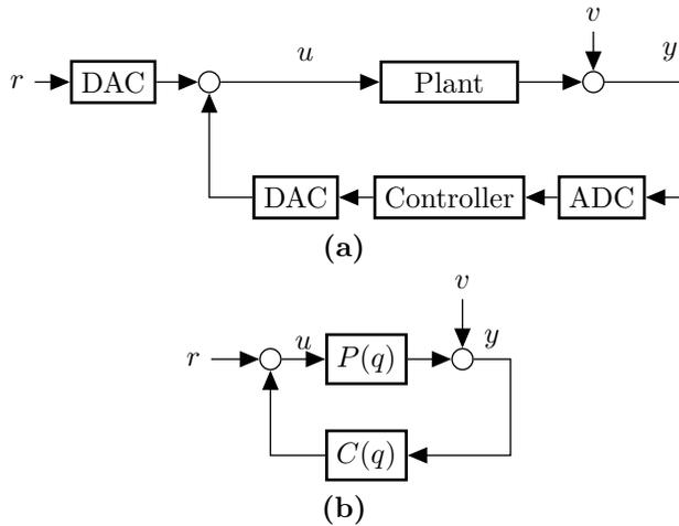
Figure 1.13: A closed-loop system as considered in the closed-loop identification literature.
