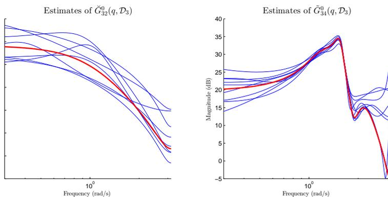
Figure 5.10: Results of Identification Experiments using the Two Stage Method as described in Example 5.31. The red lines denote the transfer functions of the immersed network for  $\mathcal{D} = \{2, 4\}$ , the blue lines denote the estimates.
