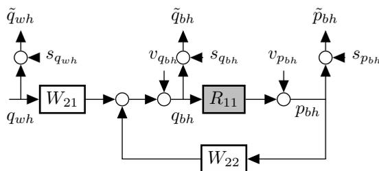
Figure 8.3: Bilaterally coupled reservoir/well bore with measurements.
