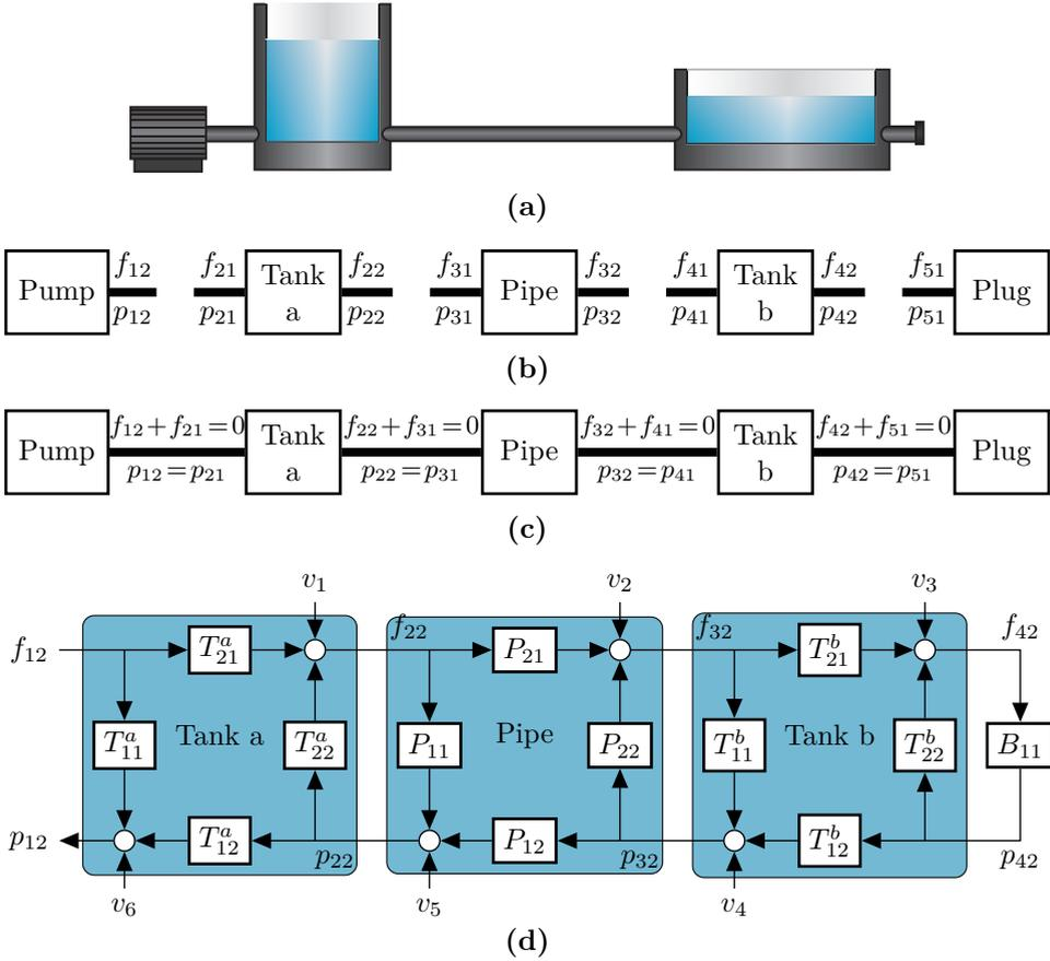
Figure 2.5: Simple hydraulic system.
