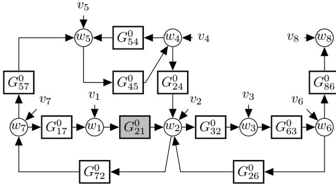
Figure 6.2: Example of a dynamic network. The sensor noise is not shown in the figure, but it is still assumed that in the available data set, each internal variable is measured with sensor noise. The labels of the  $w_i$ 's have been placed inside the summations indicating that the output of the sum is  $w_i$ .
