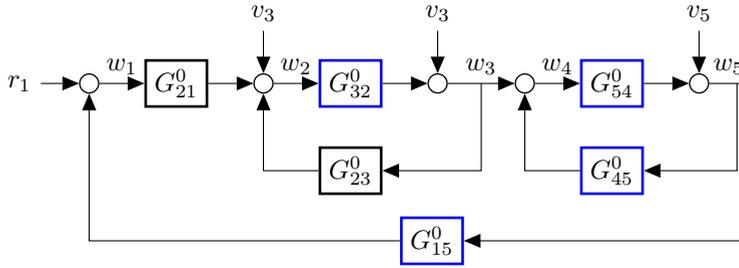
Figure 4.5: Dynamic network with 5 internal variables, of which 4 (blue-colored) transfer functions can be consistently identified using the Two-Stage Method presented of Algorithm 4.9.
