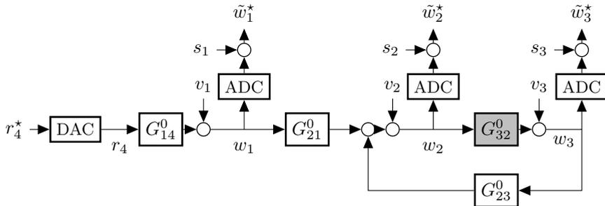
Figure 7.2: Closed loop data generating system
