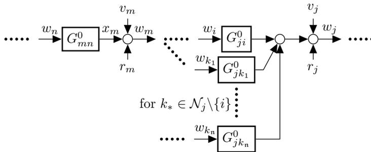
Figure 4.6: Single building block in a network structure, where the internal variable  $w_i$  is excited through a reconstructed noise variable  $v_m$ .
