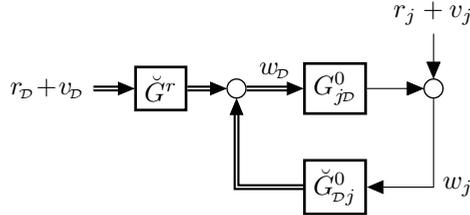
Figure 4.1: Closed Loop representation of  $w_j$ . Double lines denote multivariable paths.
