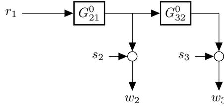
Figure 1.12: Cascaded system that is considered in Wahlberg et al. (2009); Everitt et al. (2013, 2014), where  $r_1$  denotes an external variable,  $s_2$  and  $s_3$  denote sensor noise.
