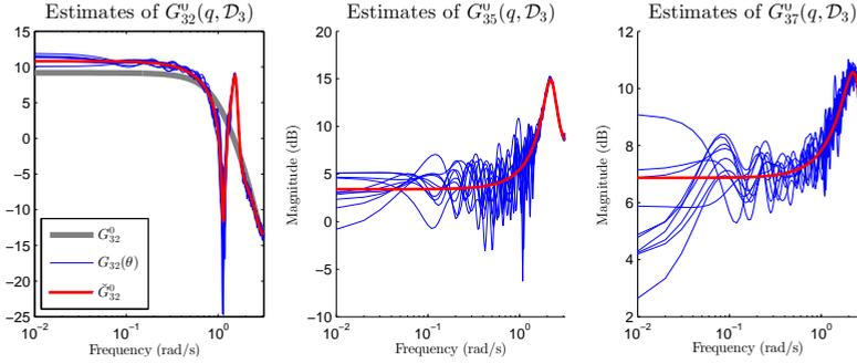
Figure 5.11: Results of Identification Experiments using the Direct Method as described in Example 5.31. The red lines denote the transfer functions of the immersed network for  $\mathcal{D} = \{2, 5, 7\}$ , the blue lines denote the estimates, and the gray line denotes the transfer function  $G_{32}^0$  of the original network.
