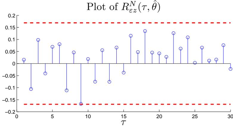
Figure 6.6: Results of the validation test presented in Section 6.7 for the setup considered in Examples 6.22 and 6.23. The red dashed lines represent the 95% confidence intervals.
