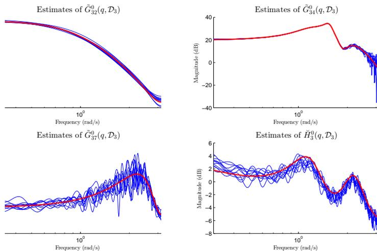
Figure 5.9: Results of Identification Experiments using the Direct Method as described in Example 5.31. The red lines denote the transfer functions of the immersed network for  $\mathcal{D} = \{2, 4, 7\}$ , the blue lines denote the estimates.
