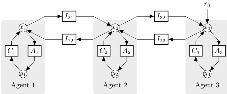
Figure 1.2: Model of the multi-agent system shown in Figure 1.1 using transfer functions. The variable  $x_i$  denotes the state of agent  $i$  (could be position and velocity for instance);  $y_i$  denotes the output of agent  $i$ ; and  $r_3$  is an external reference variable. The transfer function  $A_i$  denotes the internal dynamics of agent  $i$ ,  $C_i$  denotes the controller dynamics of agent  $i$ , and  $I_{ij}$  denotes the dynamics of the interconnection between agents.
