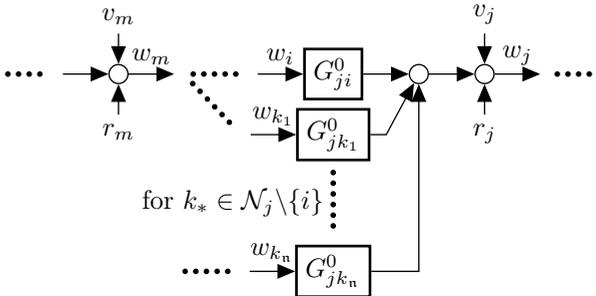
Figure 4.4: Graphical representation of a data generating system where the internal variable  $w_i$  is excited through an external variable  $r_m$ .
