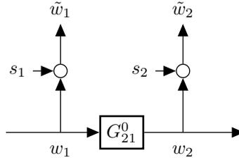
Figure 3.4: An open loop data generating system with sensor noise on both the input and the output.
