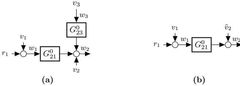
Figure 4.3: Example of a system where not all  $w_k$ ,  $k \in \mathcal{N}_j$  need to be included as inputs in the predictor ( $w_3$  can just be considered as an uncorrelated disturbance).
