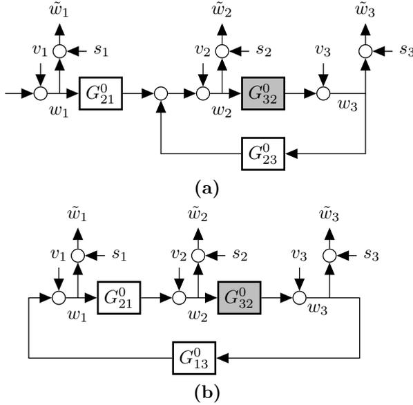
Figure 6.1: Closed loop data generating systems
