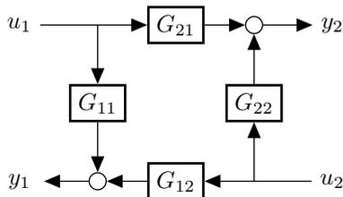
Figure 2.6: Graphical illustration of a bilaterally coupled system.
