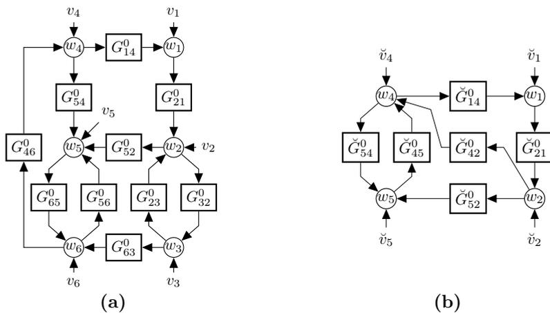
Figure 5.4: (a) Original dynamic network considered in Example 5.7. (b) Immersed network with  $w_3$  and  $w_6$  removed.
