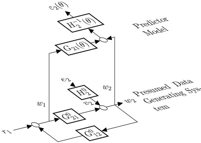
Figure 3.3: Closed-loop identification setup.
