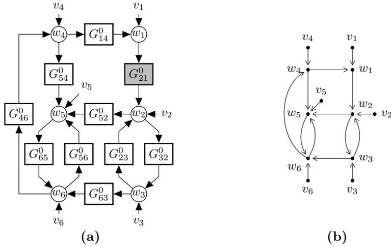
Figure 5.2: A diagram (a) and graph (b) of the network for Examples 5.4 and 5.7.
