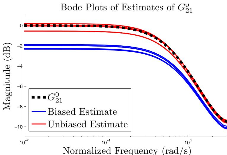
Figure 6.5: Frequency responses related to the system of Fig. 6.4:  $G_{21}^0$  (dashed), five realizations of estimated frequency responses using the Direct Method (blue) and the generalized IV Method (red).
