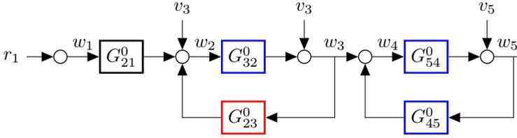
Figure 4.7: Dynamic network with 5 internal variables, of which 1 (red-colored) transfer function can be consistently identified with the two-stage method presented in this section 4.5.1 based on reconstructed noise signals.
