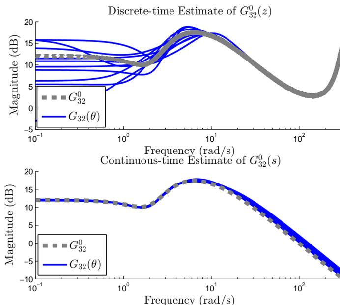
Figure 7.4: Results of direct and indirect continuous-time identification approaches for the continuous-time system shown in Fig. 7.3 with a sampling frequency of 100Hz.
