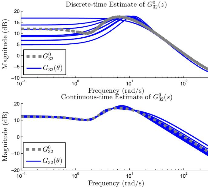
Figure 7.5: Results of direct and indirect continuous-time identification approaches for the continuous-time system shown in Fig. 7.3 with a sampling frequency of 250Hz.
