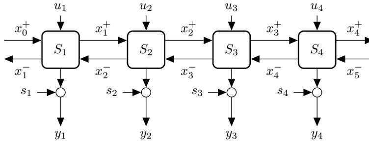
Figure 1.11: A spatially interconnected system. The  $x$ 's represent the states of each of the subsystems,  $u$ 's denote external inputs,  $s$ 's denote sensor noise which is modelled as a stochastic process with rational power spectral density, and the  $y$ 's denote the measured outputs of the subsystems.
