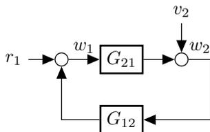
Figure 2.3: Typical closed-loop model in system identification
