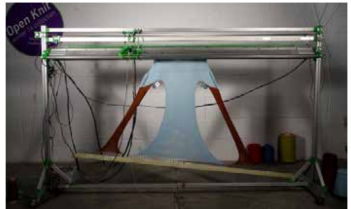
Figure 4. OpenKnit, open source knitting machine
