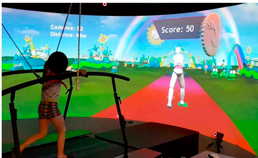
Fig. 1. Experimental set-up with treadmill and virtual reality screen (GRAIL, Motek Medical B.V., Amsterdam, Netherlands). 3D motion capture (Vicon, Oxford, UK) is integrated with virtual reality using D-Flow software (Motek Medical B.V., Amsterdam, Netherlands) to provide real-time gait analysis and visualisation. With placement of 8 markers, lower limb and trunk movements are visualised using an avatar. Intuitive biofeedback on a range of gait parameters may be attached to the avatar depending on the goal of the patient. This may include step length/width (as pictured), cadence, pelvis tilt, pelvis obliquity, hip extension and/or knee extension at initial contact. Targets for gait modification are set relative to patient baseline performance and may be adjusted by the therapist to maintain difficulty. Auditory rewards and score progression provide knowledge of results and motivation.
