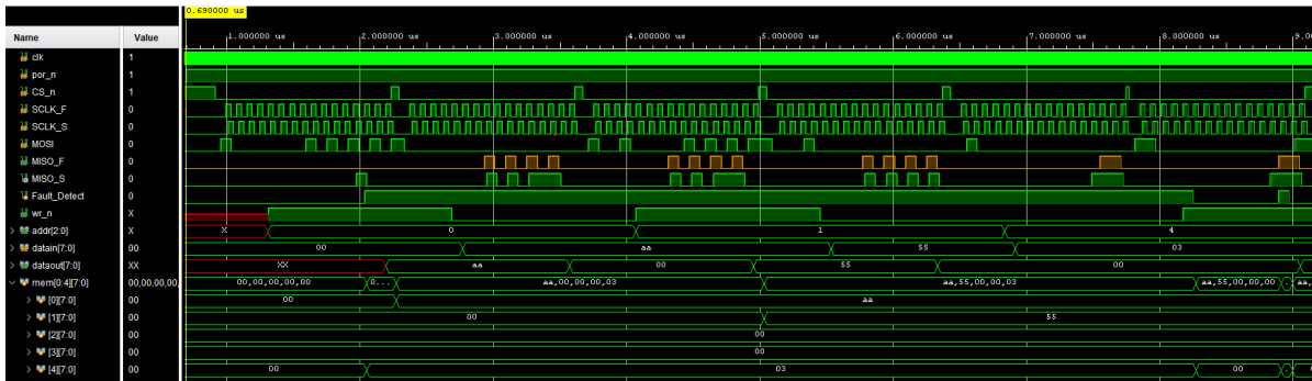
Figure 7.7: Simulation output for fault type Detected Non-Dangerous (UD), FO1 = 8'hAA, FO2 = 8'h55, CO = 8'h03
