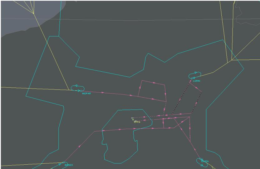
Figure 4.9: Approach paths inside the simulated TMA airspace of CDG.
