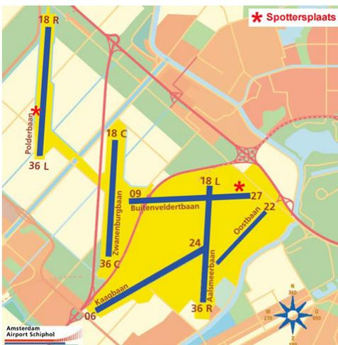
Figure 3.2: Runway configuration at Schiphol airport. Source: [www.schiphol.nl](http://www.schiphol.nl).
