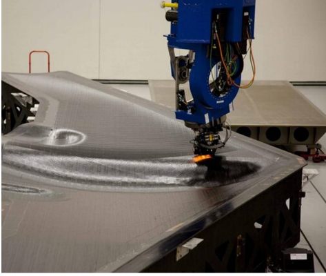
(a) AFP layup of the bottom skin of Lockheed Martin's flying wing aircraft in Palmdale, California [32].
