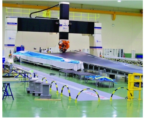
(d) MTorres ATL machine laying up of the bottom wing cover of the Airbus A350 in Illescas, Spain [35].
