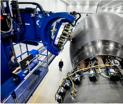
(c) ElectroImpact AFP machine laying up the front fuselage section of the Boeing B787 in Wichita, Kansas [34].
