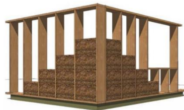
Insulation from the inside
