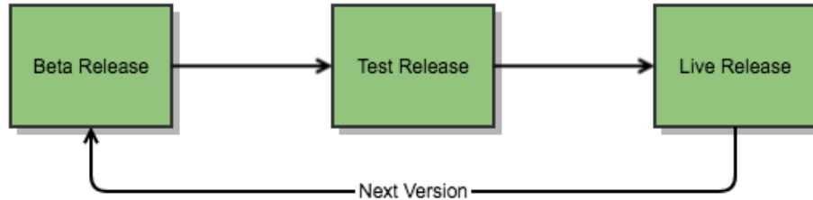
Figure 1.4: Code releases in Adyen. The first release is the Beta release where new functions are tested with artificial data. The second release is the Test release, allowing part of the users actually test the new functions. The Live release is the last one, where all users can get access to the new functions.
