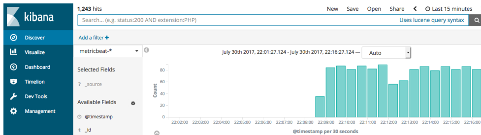
Figure 1.5: A Kibana dashboard example from Elasticsearch official website. The histograms show the frequency of a certain searching query. The details of each log entry are not shown in this example, but they are usually at the bottom of the histograms.
