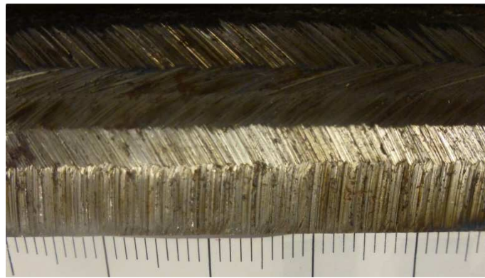
Fig. 11 Close-up of Fig. 10: heat-treated rail (gauge corner) surface roughness and facets immediately after grinding.
