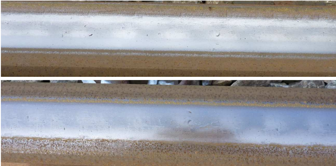
Fig. 5 Periodicity (35-36 mm; half the rail width of 70 mm) in WEL ('egg'-shaped) in the running band of R260Mn rail
