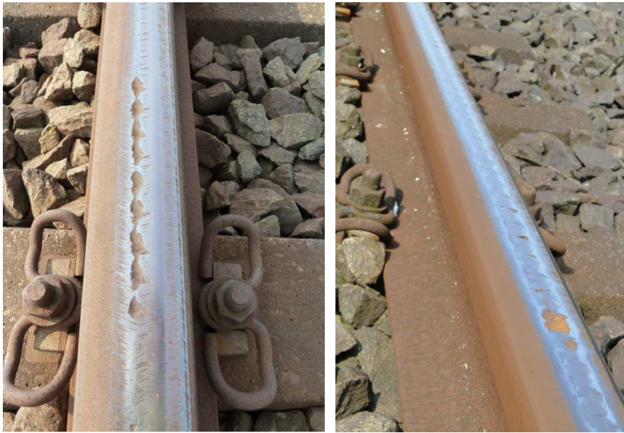
Fig. 1 Periodic spalling defects on heat-treated rail grade R370crHT/MHH
