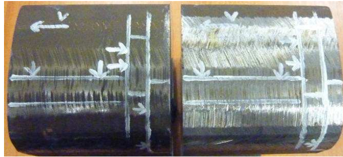
Fig. 10 Surface of heat-treated rail (R370crHT/MHH) immediately after grinding (right) and a few days of train operation (left); examined longitudinal and transverse cross-sections.
