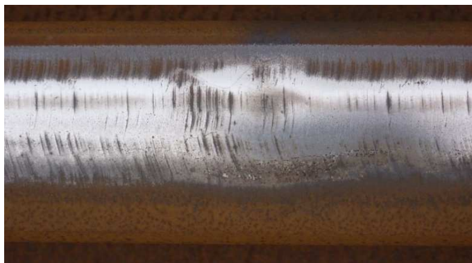
Fig. 2 A squat ground to an insufficient depth
