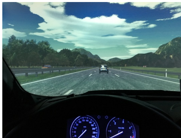
Figure 2: A take-over scenario. Participants could avoid the stationary car by steering left or right [11].
