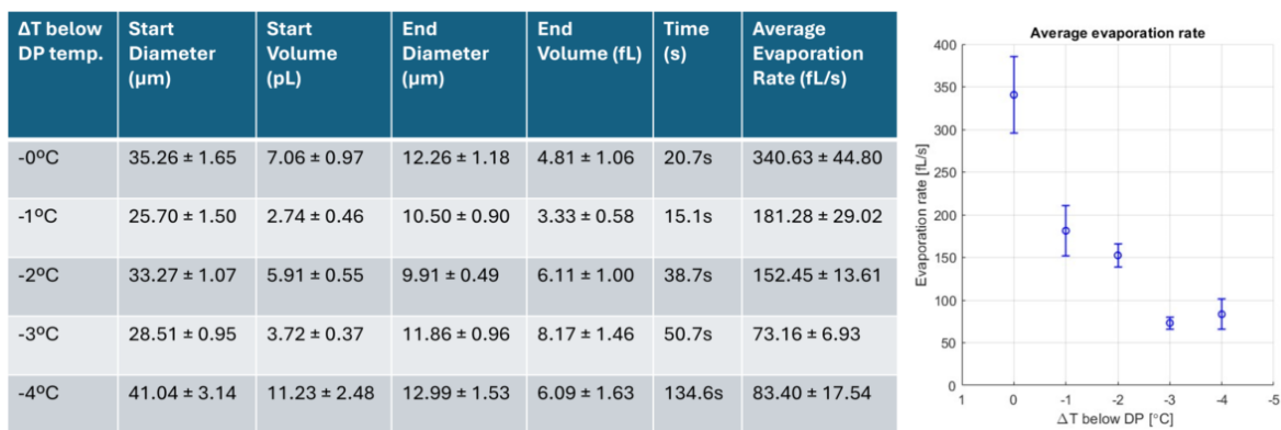
Figure 5.4: Results from measuring the average evaporation rate of five droplets on a hydrophobic EM grid at different temperature offsets below the measured dew point.
