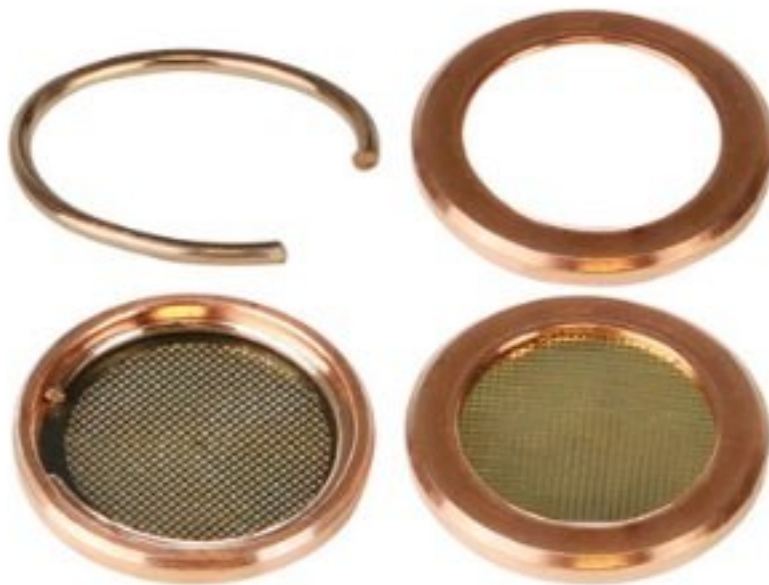
Figure 1.5: Autogrid clip and ring, clipped autogrid containing a EM grid from the front and back
