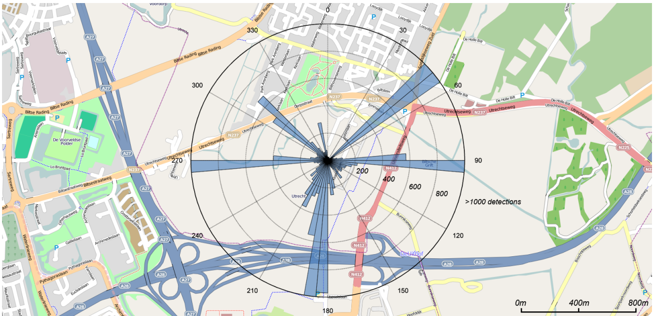
Figure 3.21: Polar histogram of the back azimuth of detections at de Bilt. All detections have Fisher ratio larger than 4 and are filtered on apparent velocity. Bins of 5 degrees width are used. Note that bins containing more than 1000 detections are limited to a length corresponding to 1000 detections. The bins from 45 to 55 degrees contain 3255 detections, from 90 to 95 degrees 13133 detections, from 185 to 190 degrees 2456 detections and from 265 to 270 degrees 3063 detections. A clear correlation is visible between the number of detections and four local sources. At 50 degrees back azimuth one finds a bicycle tunnel under the N237, at 92 degrees an overpass of the N225 over the A28, at 185 degrees a bicycle tunnel under the A28 and at 270 degrees an overpass of the A27 over the N237. The 5 story building of KNMI is located between 0 and 45 degrees back azimuth effectively blocking detections in this direction. Map source: OpenStreetMap (2009).
