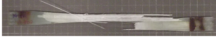
Figure 3.5: A failed unidirectional composite dog-bone coupon (TR05D13)
