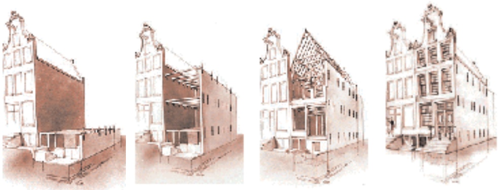
Figure 2.3 Building a Typical Amsterdam Canal-Side House
