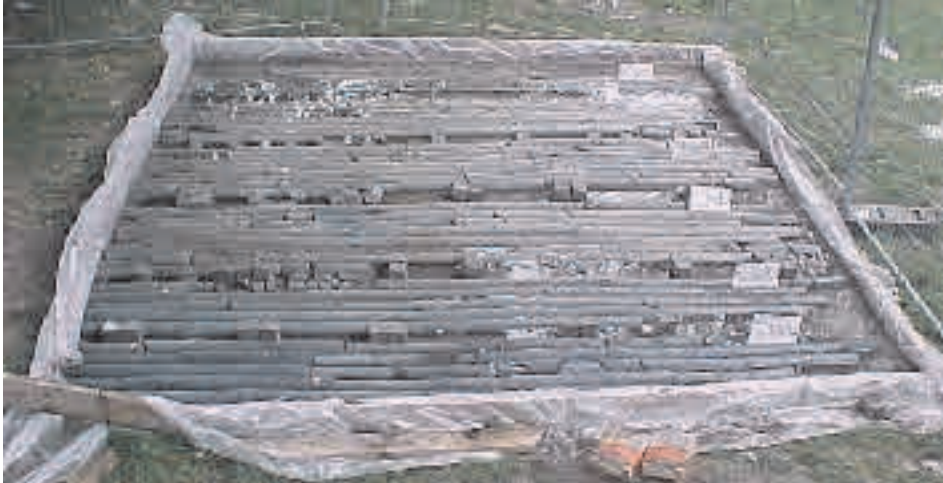
Figure 5.22 Storage in Water Basin of Cores from Jet Grouted Columns
