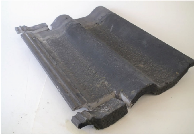
Fig. 12 Alkali-activated slag roof tile [15]
