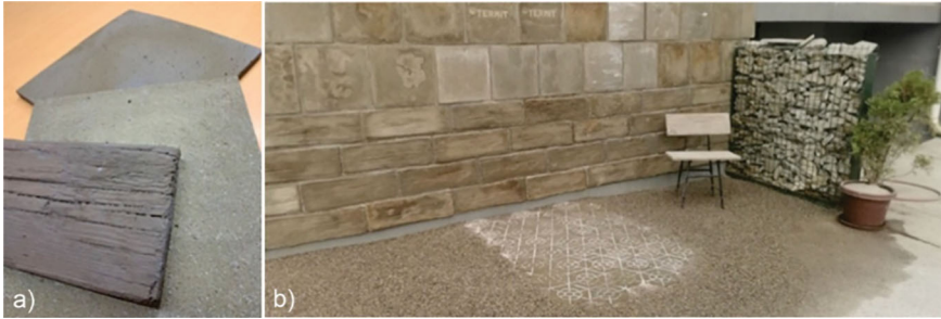
Fig. 1 a Three shapes of panels (smooth, rough and wood imitation) and b the testing field at Termit d.d [3]. Foto archive of ZAG and Termit
