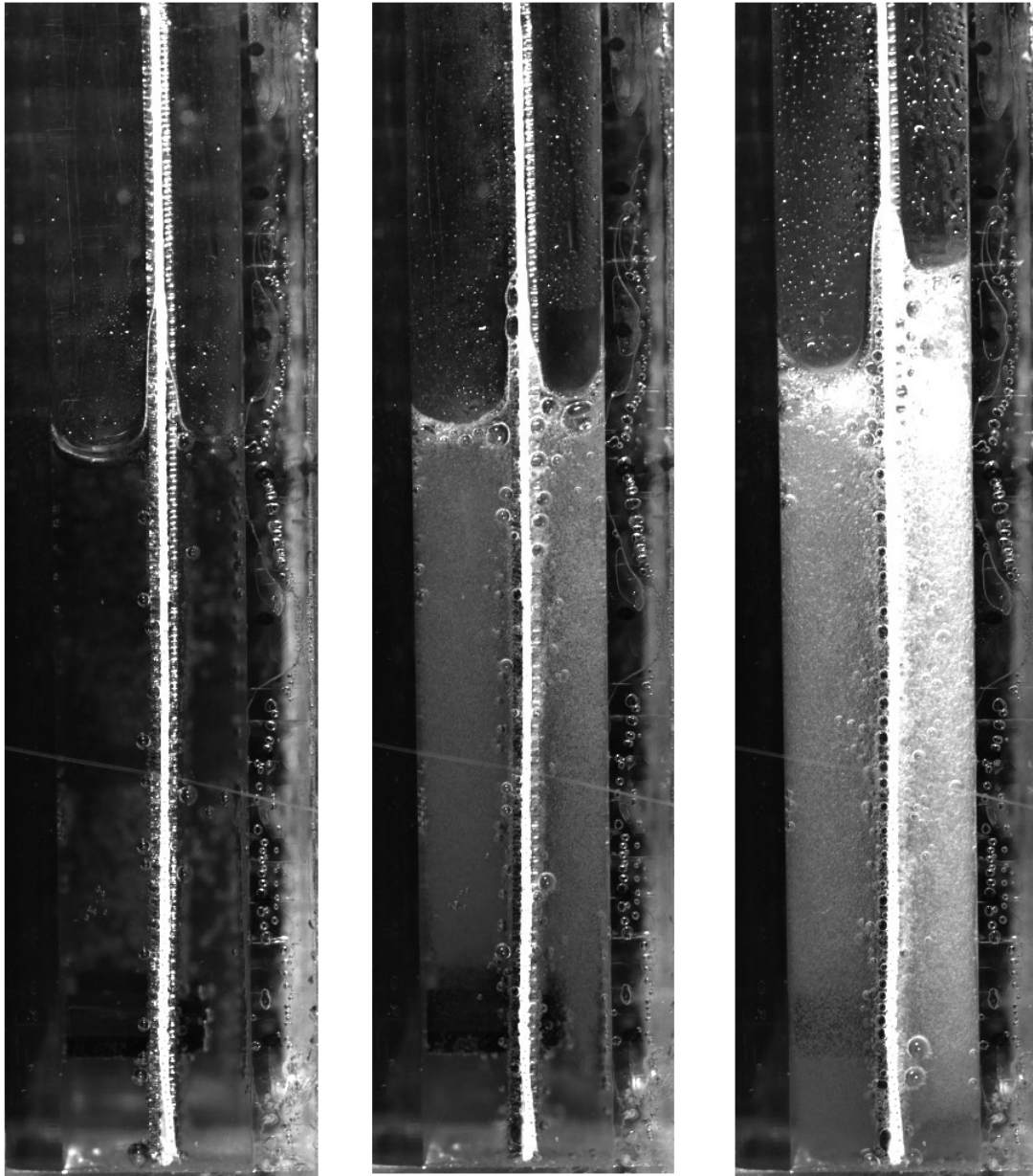
Figure A.1: Gas evolution in channels. Anodic (electrode-wall distance 6 mm) and cathodic (electrode-wall distance 5 mm) side at the left and right of the membrane respectively. Current densities of 100 (left), 1000 (middle) and 6000 A/m 2 .
