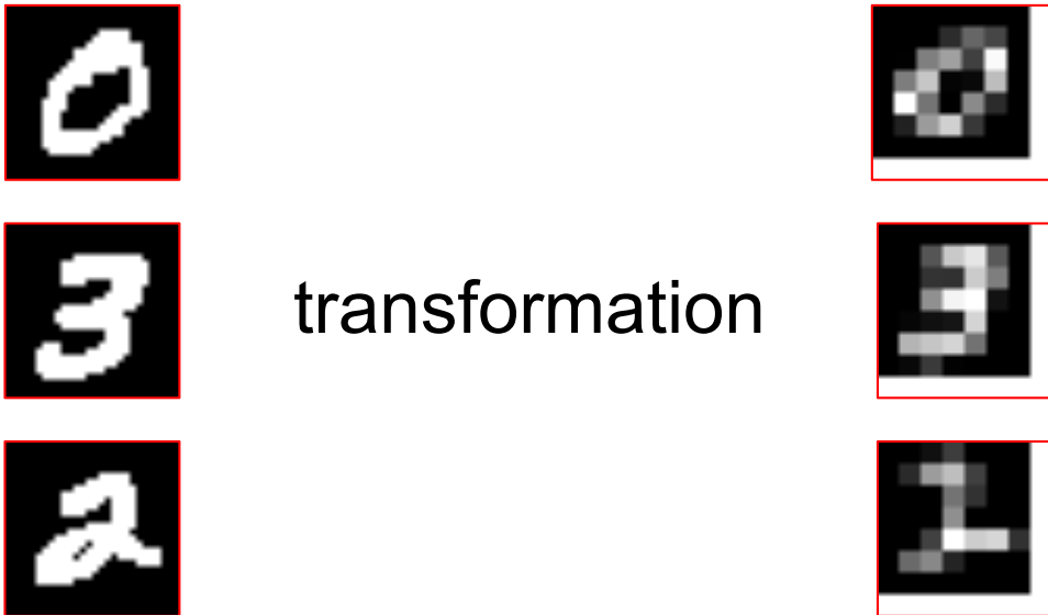
Figure 6.15: Images from the database NIST are 28x28 pixels. They were transformed into 7x7 images just by adding the light intensity that should be measured by the sensor. The last rank and column are set to 1 to implement the bias.
