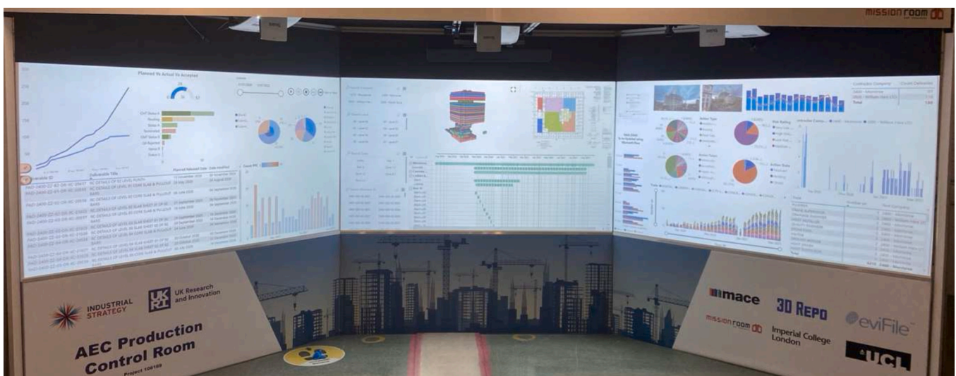
Fig. 10. Control room as an interface to the construction digital twin.
