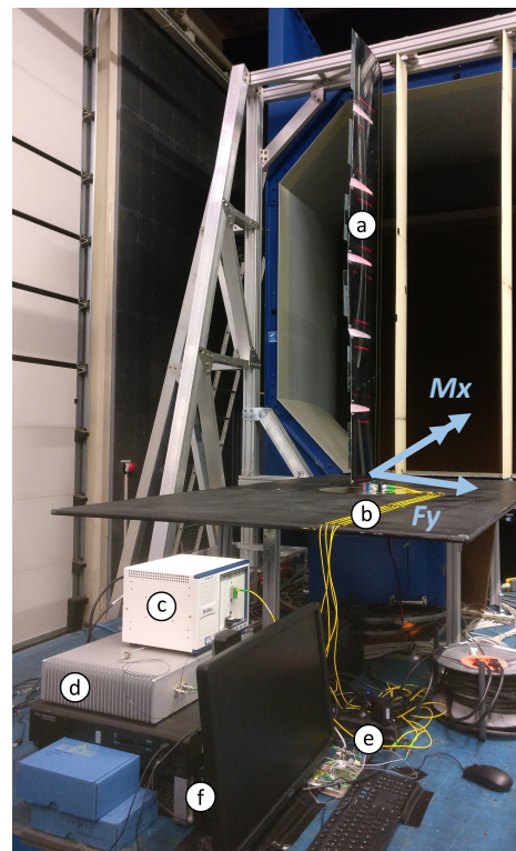
Figure 5. The experimental setup at the OJF (Open Jet Facility) low speed wind tunnel, showing the (a) wing, (b) optical fibers (yellow), (c) National Instruments interrogator, (d) Optics11 interrogator, (e) Thorlabs optical switch, and the (f) Data acquisition system.
