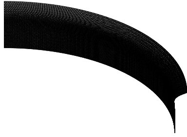
Figure 2.35: A-8 cylindrical shell: pre-buckling solution q_0
